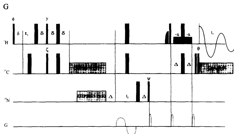
Fig. 15. Pulse schemes for through-bond correlations of amino/imino and non-exchangeable protons. (A) The 2D H(NC)-TOCSY-(C)H experiment, used to connect imino to H8 protons in guanosines [151]. The indirect detection period t_1 (see below) was partially concatenated with the first ^1\text{H} - ^{15}\text{N} INEPT using the time-shared evolution procedure, which allows a reduction of 5 ms for the longest t_1 value [234]. For the first t_1 point, \epsilon_1 = \epsilon_2 = 0.5*(dw/2 - (4\pi)PW90(^1\text{H}) - PW180(^{15}\text{N})) and \epsilon_3 = \tau_1 . For subsequent t_1 points, \epsilon_1 was incremented by dw/2 - t_1/(n+1) and \epsilon_2 was decremented by t_1/(n+1) , where dw is the dwell time and n is the total number of complex points in t_1 . The t_1 and t_2 delays were set to 2.5 and 1.25 ms respectively. The magnetization was transferred from ^{15}\text{N} to ^{13}\text{C} by cross polarization using a 44.9 ms DIPSI-3 sequence [235–237] at an rf field of 1.9 kHz. A 37.8 ms FLOPSY-8 sequence [238] at an rf strength of 5 kHz was used for the ^{13}\text{C} homonuclear TOCSY period [239]. Unless otherwise noted, all pulses have phase x . The phase cycle was \phi_1 = 2(y + 45^\circ), 2(-y + 45^\circ) ; \phi_2 = y, -y ; \phi_3 = 4(y), 4(-y) ; \phi_4 = 8(x), 8(-x) and receiver = x, 2(-x), x, -x, 2(x), -x . Instead of phase cycling \phi_2 , the two 90^\circ ^{15}\text{N} pulses before the ^{15}\text{N} - ^{13}\text{C} cross polarization can be eliminated and the phase of the ^{15}\text{N} DIPSI-3 can be phase cycled ( x, -x ) using the same receiver phase cycling as before [240]. Eliminating these two 90^\circ ^{15}\text{N} pulses should lead to a slight improvement in sensitivity for probes with low ^{15}\text{N} B1 homogeneity. The ^{15}\text{N} frequency was set to 146 ppm during the ^1\text{H} - ^{15}\text{N} and ^{15}\text{N} - ^{13}\text{C} transfers and it was shifted to 195 ppm at point a to decouple N7 and N9 during the acquisition period. The ^{13}\text{C} frequency was positioned at 151 ppm for the ^{15}\text{N} - ^{13}\text{C} hetero-TOCSY period and was shifted to 145 ppm at point a for the ^{13}\text{C} -TOCSY period and to 142 ppm at point b . To avoid a complete inversion of the water signal by the second ^1\text{H} 90^\circ pulse, the phase of \phi_1 was shifted by 45^\circ and the ^1\text{H} carrier was set to the water frequency. Radiation damping returns the water magnetization to the +z axis during the ^{15}\text{N} - ^{13}\text{C} cross polarization and ^{13}\text{C} -TOCSY periods. At point b , water flip-back is achieved with a 2.9 ms selective E-BURP pulse [241,242]. During the last INEPT periods, a WATERGATE sequence is applied to suppress the residual water signal using two 1.55 ms soft square pulses [243]. The phases of the selective E-BURP and soft square pulses were adjusted with a small angle phase shifter for optimal solvent suppression. During the detection period, ^{13}\text{C} and ^{15}\text{N} GARP1 decoupling was used at rf fields of 1.6 and 1.14 kHz, respectively. All gradients were applied along the z axis, with g_1 = 12 G/cm, g_2 = 24 G/cm and g_3 = 32 G/cm. The gradient times for g_1, g_2 and g_3 were 300, 300 and 450 \mu\text{s} , respectively. Each gradient was followed by a recovery time of 200 \mu\text{s} . (B) The uridine optimized 2D H(NCCC)H experiment employed a refocused INEPT sequence for the ^1\text{H} - ^{15}\text{N} transfer [150]. The ^1\text{H} carrier is placed at the center of the imino proton region (13.2 ppm for uridine) at the beginning of the experiment and shifted to the water frequency at point a . A 90 ms DIPSI-3 ^{13}\text{C} - ^{15}\text{N} hetero-TOCSY mixing period was used at an rf field strength of 1.9 kHz, using ^{13}\text{C} and ^{15}\text{N} carrier frequencies of 169 and 160 ppm, respectively. The ^{13}\text{C} carrier was shifted to 139 ppm at point a . Water magnetization returns to the +z axis by radiation damping during the ^{13}\text{C} - ^{15}\text{N} hetero-TOCSY period. After this ^{13}\text{C} - ^{15}\text{N} hetero-TOCSY period, the magnetization is transferred from C4 to H6 using a string of concatenated ^{13}\text{C} - ^{13}\text{C} and ^{13}\text{C} - ^1\text{H} INEPT type transfers. The second half of the ^{13}\text{C} - ^1\text{H} reverse INEPT transfer has been adapted to include a WATERGATE solvent peak suppression [243]. In this scheme the proton 90^\circ pulse in the center of the reverse INEPT period is preceded by a selective water flip-back 90^\circ E-BURP pulse (2.8 ms) at point b [241,244]. In the final refocused INEPT interval, the proton 180^\circ pulse is flanked by two square 1.67 ms 90^\circ pulses of phase -x , and the carbon 180^\circ pulse is placed at the interval t_1 = 1/(4*J_{\text{CH}}) following the proton 90^\circ pulse. The phases of the selective square 90^\circ pulses and the 90^\circ E-BURP pulse are further optimized for maximum solvent peak suppression, using a small angle phase shifter. The transfer delays were \tau = 3.6 ms, \tau_1 = 2.5 ms and \tau_2 = 1.25 ms. G_z denotes the z axis pulsed-field gradients with the following values: g_1 = 300 \mu\text{s} at 24 G/cm and g_2 = 450 \mu\text{s} at 32 G/cm. A 400 \mu\text{s} recovery time was added after each gradient. Quadrature detection in the proton t_1 period was obtained with the TPPI-States method [245]. The 16-step phase cycle is \phi_1 = x, -x ; \phi_2 = y, y, -y, -y ; \phi_3 = 4(x), 4(-x) ; \phi_4 = 8(x), 8(-x) and receiver = 2(x, -x, -x, x), 2(-x, x, x, -x) . (C) The cytidine optimized 2D H(NCCC)H [150], where the ^{13}\text{C} - ^{15}\text{N} refocused INEPT period in the pulse sequence given in (B) is replaced with a ^1\text{H} - ^{15}\text{N} hetero-TOCSY period. A 7.5 ms half DIPSI-3 (R, -R supercycle) sequence [237] was used for the ^1\text{H} - ^{15}\text{N} hetero-TOCSY transfer at an rf field of 1.9 kHz with the ^{15}\text{N} carrier set to 96.7 ppm and the ^1\text{H} carrier before point a set to 7.6 ppm. Other changes compared to the pulse sequence given in (B) were that the ^{13}\text{C} - ^{15}\text{N} hetero-TOCSY period was set to 45 ms ( J_{\text{NC}} \approx 20 Hz for cytidine instead of \approx 10 Hz for uridine) and an eight-step phase
